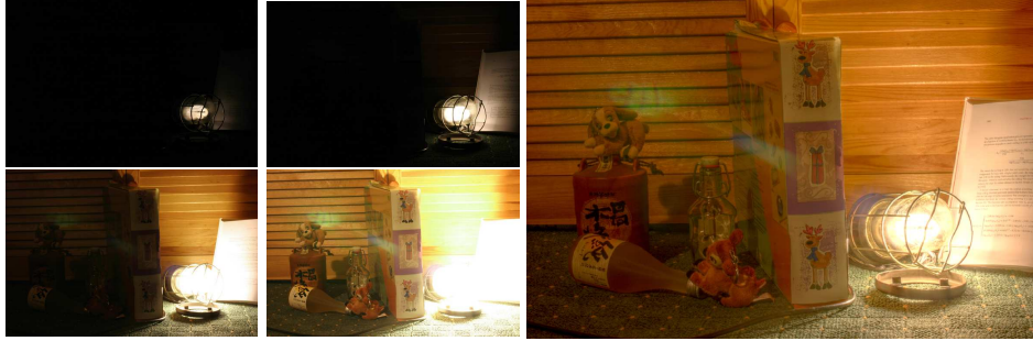
Figure 3. Four LDR images selected from a sequence of photographs used to build an HDR image. The resulting HDR image (right) was created by the pfshdrcalibrate and, to display in LDR media, tone mapped using contrast domain operator. 23
