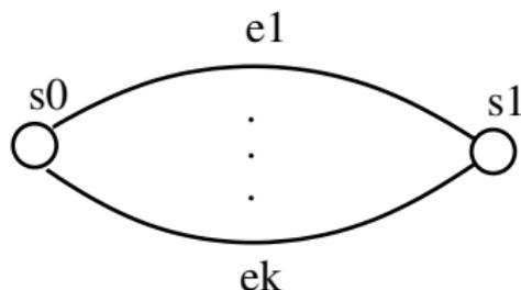
parallel links with lengths  $L_1 < L_2 < \dots < L_k$
