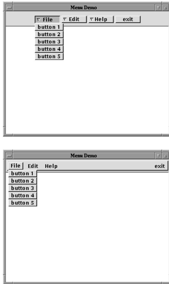
**Figure 11.17** Menu buttons: The upper screenshot shows the default style and the lower screenshot shows the menu bar style.
