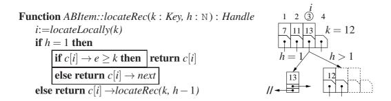
Figure 1: Corrected version of function *locateRec* for (a,b)-trees. The framed pieces are new.
