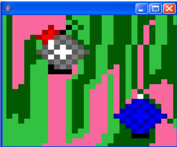
Figure 7 : Simulation of Robot movements in Java where the pink, light green and dark green areas represent the paths traversed by 3 different robots and red, grey and blue represent the areas where different smell were found.
