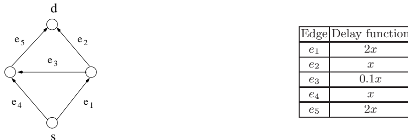
Fig. 5. A counter-example to show that \mathcal{P}_h can be a strict subset of all s - d paths in G(V, E') .
