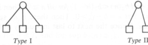
FIG. 8. The subtrees in the fringe of a 2-3-tree.
