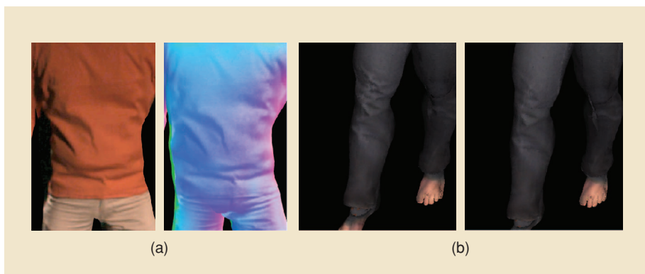
[FIG9] (a) Comparison between an input frame and the corresponding normal map that we reconstructed. For rendering, the three components of the surface normals were encoded in the three color channels. One can see that subtle surface details have been captured at high accuracy. This level of accuracy also enables us to (b) faithfully reproduce time-varying geometric details, such as the wrinkles in the trousers around the knee.
