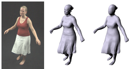
Figure 9: Input frame (l) and reconstructions using a detailed (m) and a coarse model (r). Although the fine details on the skirt are due to the input laser scan (m), even with a coarse template, our method captures the folds and the overall lifelike motion of the cloth (r).
