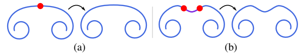
Figure 3: Segment Merge Criteria. Pre-merge segment boundaries are colored (\bullet) , and two different average segment orientations are colored (\circ) and (\circ) . (a) A pair of segments is mergeable if they both have similar average orientations. (b) A triplet of segments is mergeable if the center segment (\circ) has a low average total curvature compared to its neighboring segments, which have similar average orientations.
