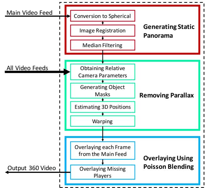
Figure 1: The 3 stages of our immersive content generation technique, and their main components.
