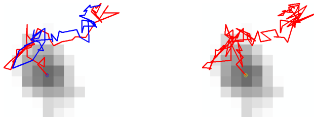
Figure 1. Tracking with \Delta x^2 + \Delta y^2 (left) and \Delta x^2 + \Delta y^2 + \Delta t^2 (right). Two interleaved tracks are produced for one molecule on the left, whereas there is exactly one on the right. The background images are inverted for better readability.
