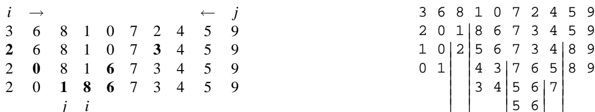
Figure 2: Execution of qSort (Fig. 1) on (3, 6, 8, 1, 0, 7, 2, 4, 5, 9) using the first element as the pivot and n_0 = 1 . The left-hand side illustrates the first partitioning step, showing elements in bold that have just been swapped. The right-hand side shows the result of the recursive partitioning operations
