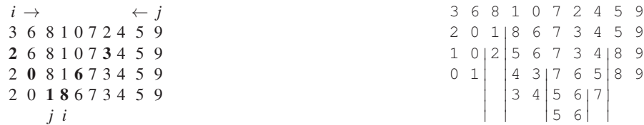
Fig. 5.10. Execution of qSort (Fig. 5.9) on \langle 3, 6, 8, 1, 0, 7, 2, 4, 5, 9 \rangle using the first element as the pivot and n_0 = 1 . The left-hand side illustrates the first partitioning step, showing elements in bold that have just been swapped. The right-hand side shows the result of the recursive partitioning operations.
