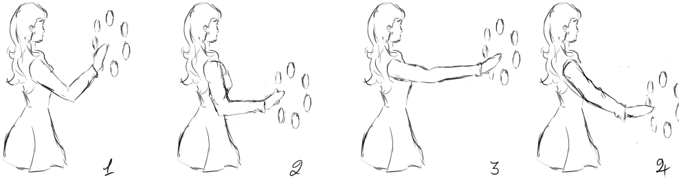
FIGURE 5.1: Four interaction zones used for determining the best model. 1) Target is shoulder height and arm is bent. 2) Target is waist height and arm is bent. 3) Target is shoulder height and arm is straight. 4) Target is waist height and arm is bent.
