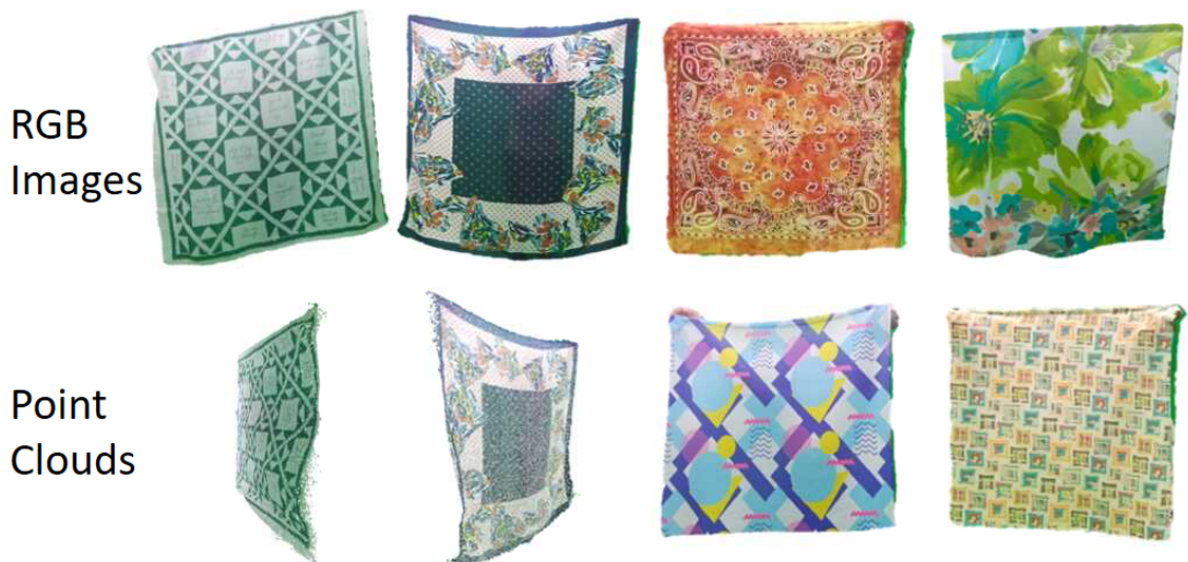
Figure 4.1: We record a new real “ \phi -SfT dataset” of nine sequences with reference depth data to facilitate quantitative comparisons of monocular 3D surface reconstruction methods. Our setup consists of a synchronised RGBD camera. The depth camera is used to extract point clouds that serve as pseudo-ground-truth for evaluation.
