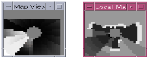
Figure 3: Sonar scans with learned (l) and manually designed (r) sensor model (darker color means lower occupancy probability)
