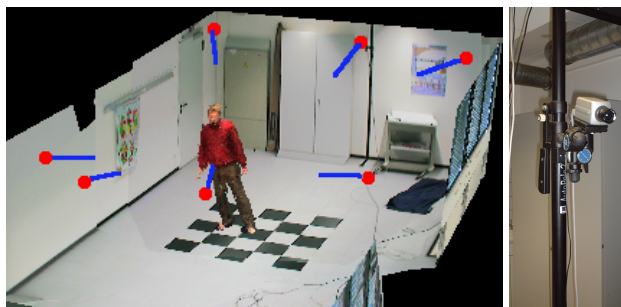
Figure 1: The figure on the left shows an example seven-camera setup used in our system. The red spheres denote camera positions and their viewing directions are shown as blue lines. The image on the right shows one of the video cameras used.
