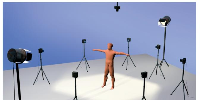
Fig. 3. Illustration of camera and light source arrangement.
