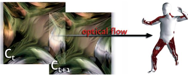
Fig. 4. Detection of relative cloth shift between two subsequent combined textures  $C_t$  and  $C_{t+1}$  (in parameterization II) by means of optical flow. Areas where shifting textiles were found are marked in red on the 3D model.
