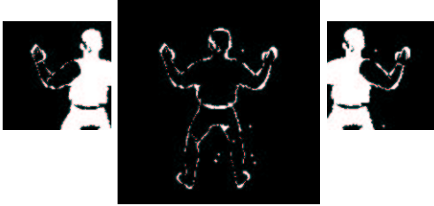
Figure 3: Global energy function (center) and smaller sub-windows (128x128 pixels) used to optimize the arm positions (shown for one camera).
